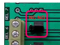
Rel X – relay output for fire condition № X, where X is from 1 to 2 C – common contact NO – normally open contact NC – normally closed contact
