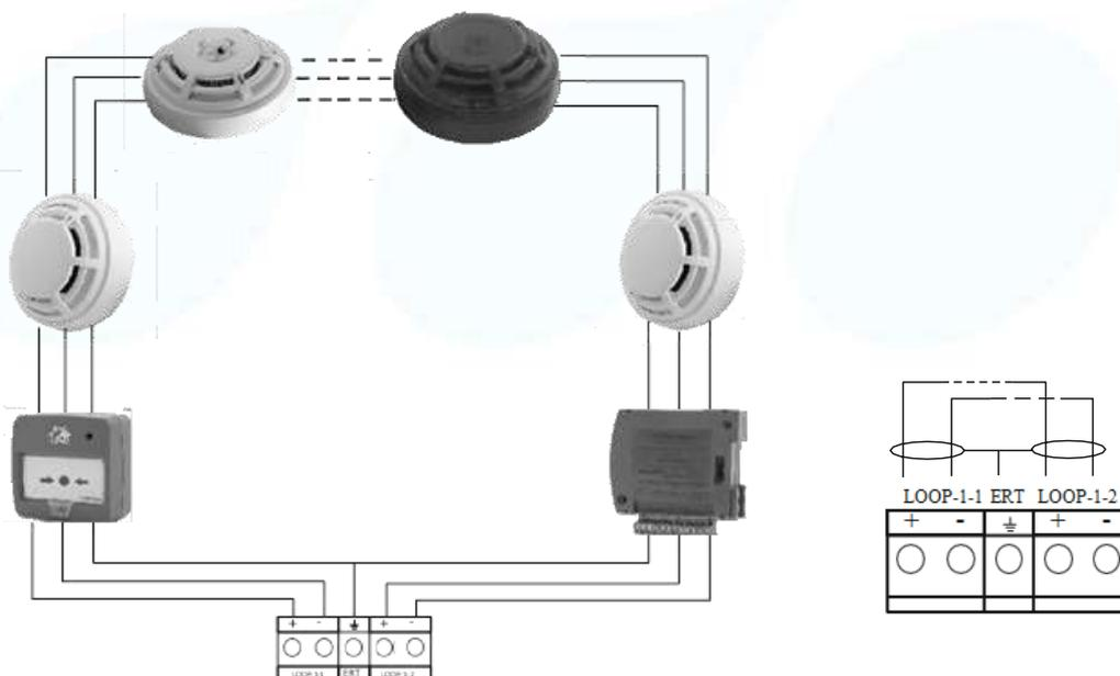
Fig. 7 - Example of devices connected in a loop
