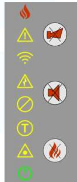
**5.2.2. Initial screen of the panel** – in Fig. 2 is shown the homescreen with the characteristic information areas and function buttons.
